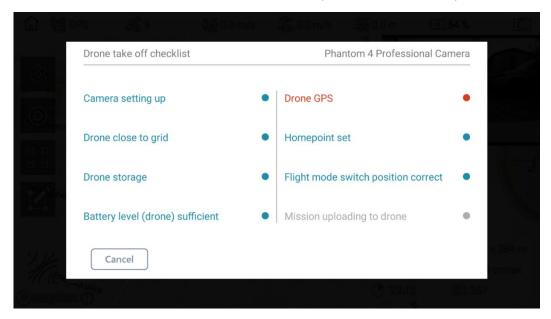
III. Drone close to grid error – If the missions start/end point is further than 200m or end/start point is further than 1000m, move your drone closer to selected area or reduce the mission.
